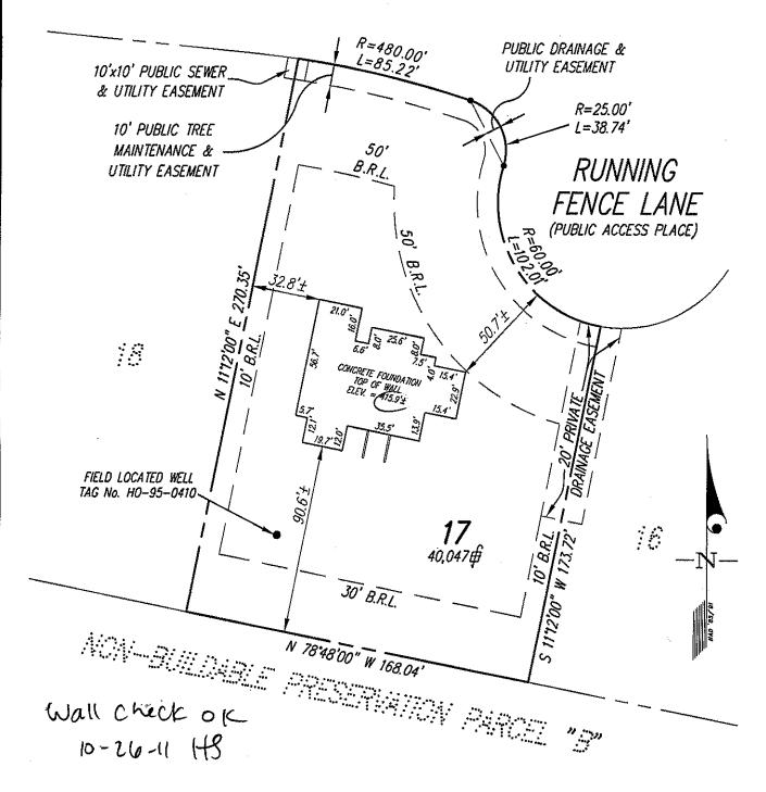
BUILDING SETBACKS (B.R.L.'s) SHOWN HEREON PER PLAT No. 19226 SETBACK DISTANCES SHOWN HEREON AS "±" HAVE AN ACCURACY OF ±0.1' FOOT.
