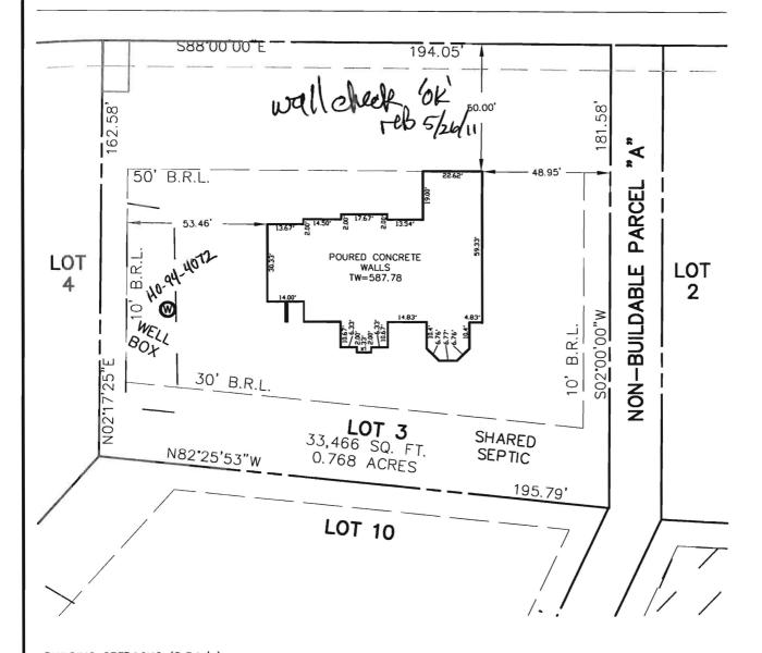
BUILDING SETBACKS (B.R.L.'s) SHOWN HEREON PER SITE DEVELOPEMENT PLAN SETBACK DISTANCES SHOWN HEREON AS "±" HAVE AN ACCURACY OF ±0.1' FOOT.
