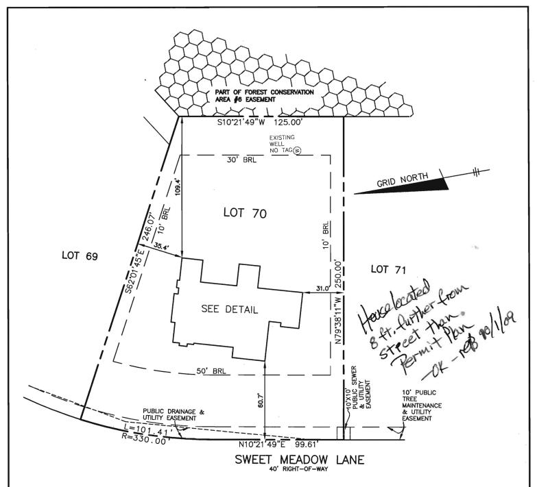
TOP OF FOUNDATION WALL ELEVATION = 413.1' OFFSET DIMENSIONS TO PROPERTY LINES ARE  $\pm$  0.2'
