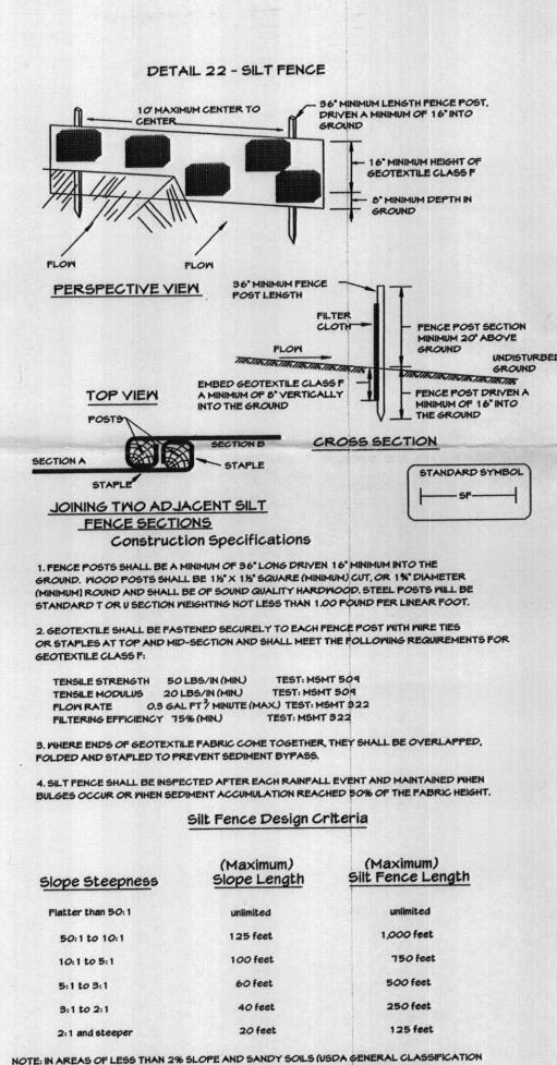
SYSTEM, SOIL CLASS A) MAXIMUM SLOPE LENGTH AND SILT FENCE LENGTH WILL BE UNLIMITED. IN THESE AREAS A SILT FENCE MAY BE THE ONLY PERIMETER CONTROL REQUIRED
