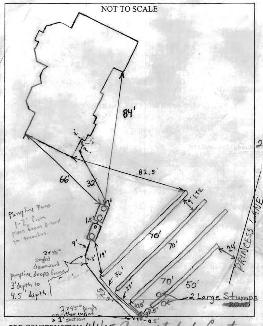
TRENCH/DRAINFIELD DATA WIDTH INLET, BOTTOM 3' 4,5 7
