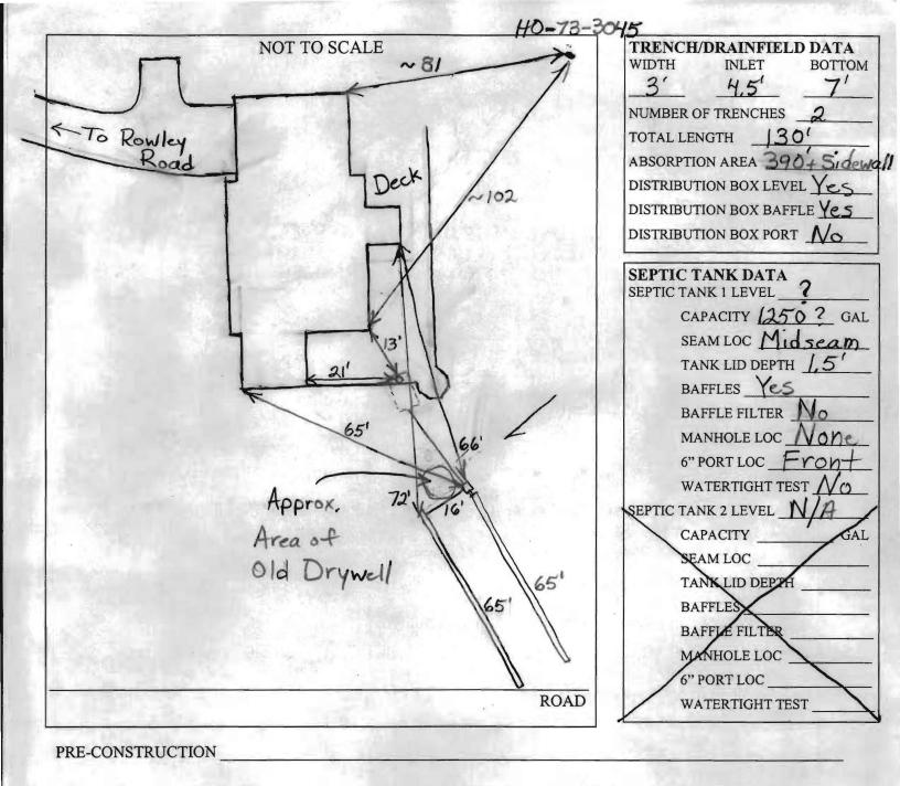
INSTALLATION 4/18/05 Old drywell pumped out and filled with dirt. Pear tank baffle replaced. Irenches installed as per spece. on Pobert Lyocks permit, BB FINAL INSPECTOR B. Baber DATE OF APPROVAL 4/18/05
