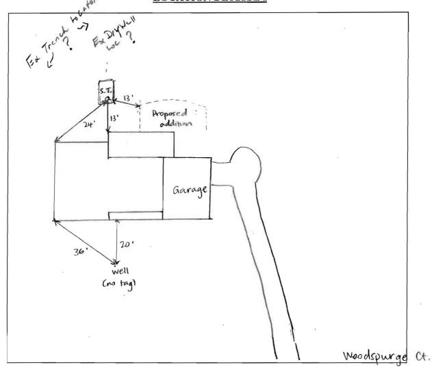
COMMENTS: Contractor and owner on site Incated cleanant and edge of septic tank closest to stake for addition - 13' from corner of tank to addition. Owner says dry well was abandoned when trench was installed and no other tanks on property. Tried to probe but ground was hard. Located well-owner says 11's the original, 90' deep and good yield. No other wells on property.
