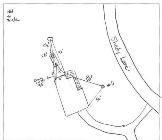
comments: Site insp. contractor not on site spoke to contractor will add man hole to septic tank wiriser, replace line from tank to abox to make fall, add site clean out to abox, add speedy levelers to abox and shot down failing trench and add observation pipe to lower trench which is still operational DATE: 4 19/18 INSPECTOR: R. Roppe port
