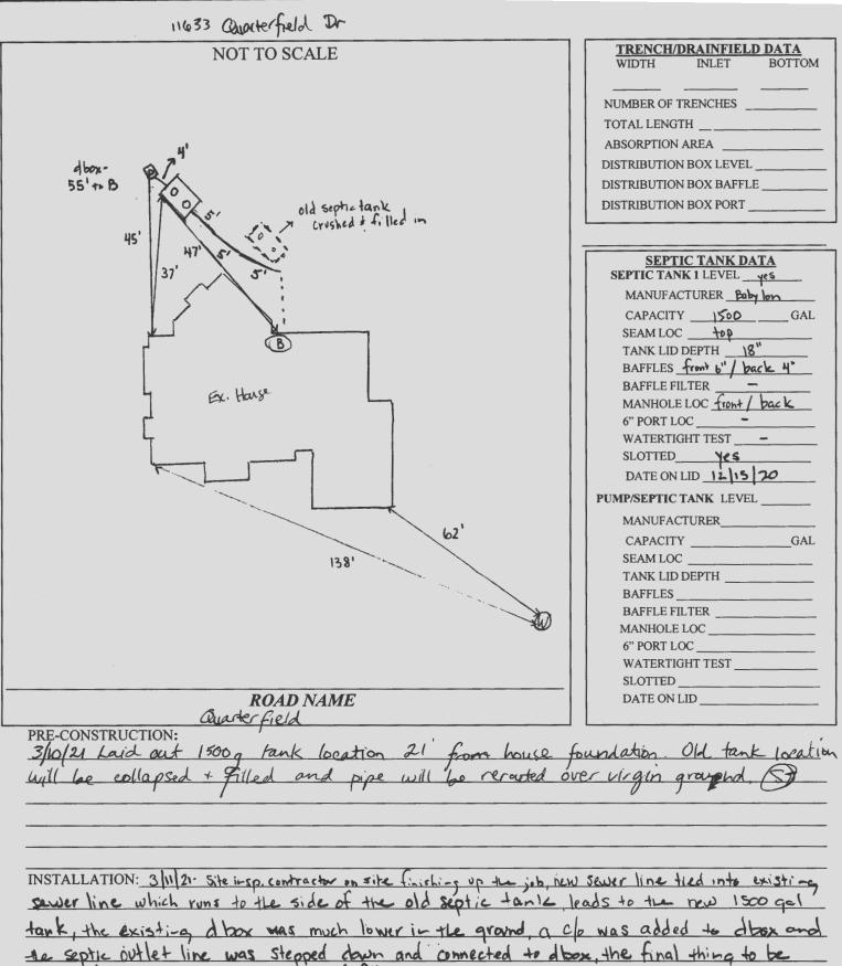
completed is - collapsing the old tank and filling it in contractor stated that it'd done befit he left the site (Jamie), ok to continue is backfill
