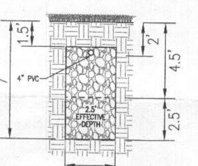
FIRST REPLACEMENT & SECOND REPLACEMENT SYSTEM TRENCH DETAIL
