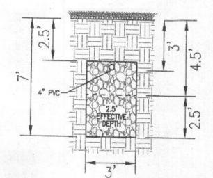
INITIAL SYSTEM TRENCH DETAIL NOT TO SCALE
