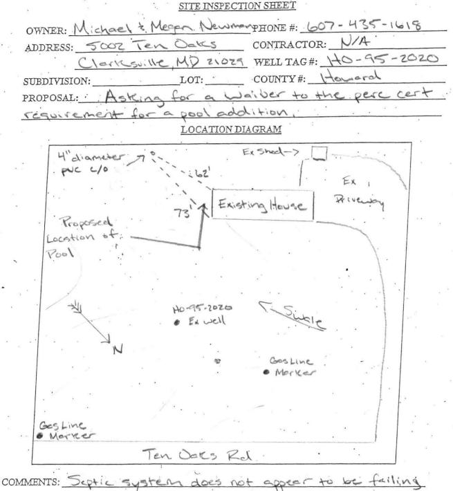
COMMENTS: Septic system doe's not appear to be failing to the surface. Could open 1/0. but could not see anything inside. Well appears to be in good condition. Secure Zpe cop and well tag the are on the well. Well has been GPS Located. DATE: 6/10/2019 INSPECTOR: RSF
