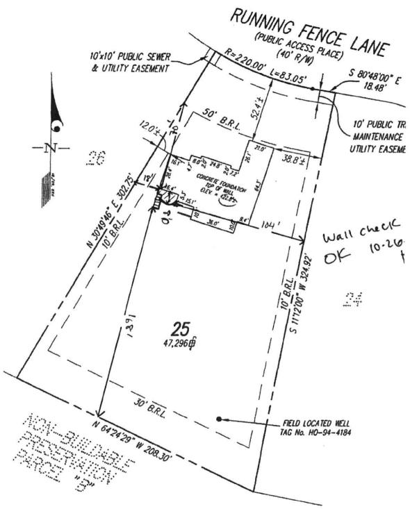
BUILDING SETBACKS (B.R.L.'s) SHOWN HEREON PER PLAT SETBACK DISTANCES SHOWN HEREON AS "±" HAVE AN ACCURACY OF ±L
