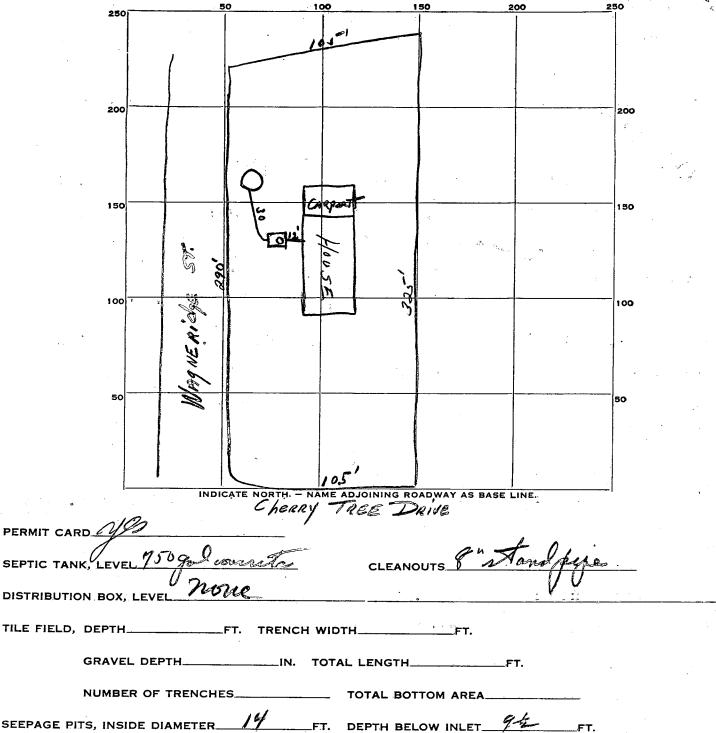
TILE FIELD, DEPTH\_ NUMBER OF TRENCHES\_\_\_\_\_ SEEPAGE PITS, INSIDE DIAMETER 14 FT. DEPTH BELOW INLET 94 FT. ABSORBENT AREA\_\_\_\_\_SQ. FT. REMARKS\_ INSPECTOR
