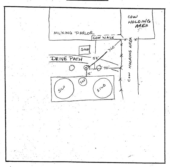
COMMENTS: 7/28/94 Avaliable AREA limited - well to be furthest distance from cow holding area as possible. ( collapsing-replacement needed immediatly DATE: INSPECTOR: Amy Mc Miller
