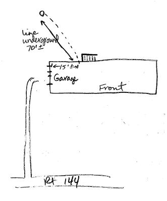
9-14-87 Pitless at 32 inches. Well line covered. No ground; Plastic casing. Connection into house covered on outside. House connection de inside, Pitless is marginal. DK. LE Nadean
