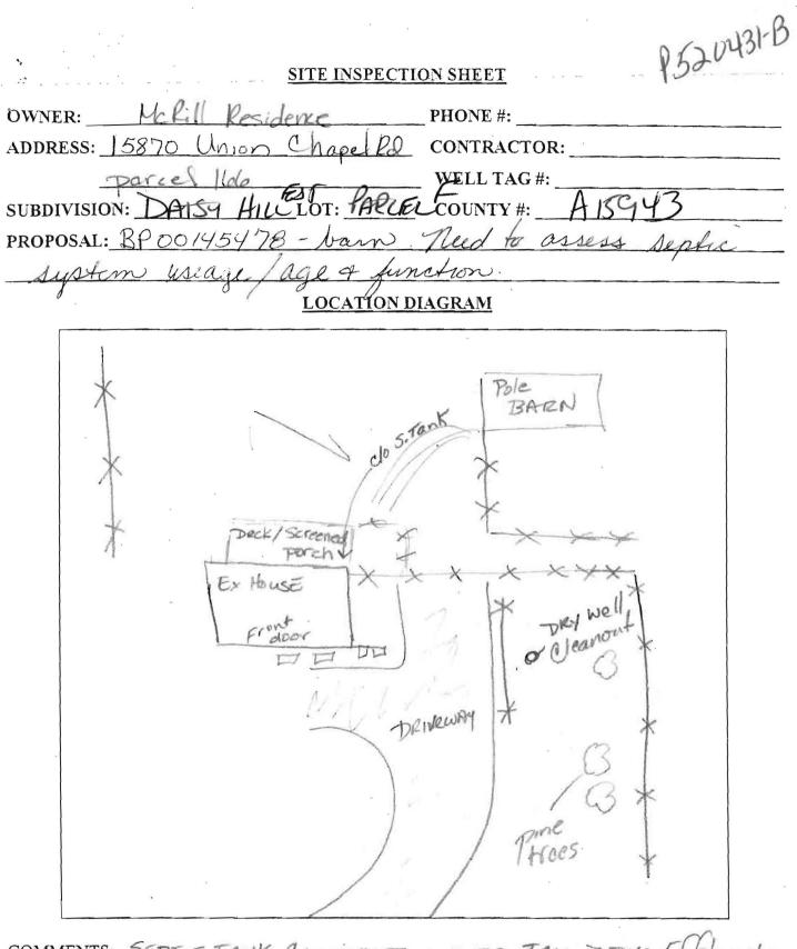
COMMENTS: SEDTIC TANK CLEANDUT UNDER TALL DECK. APPORT 31/2 below grade, evel The dry Approx 4' below grade. Previous specs require Nuner In bedrooms. Repair + upgrade States house 4 needed Mas DATE: 12/24/03 INSPECTOR: pontan A acce \* NEED to Verify well tag # & location
