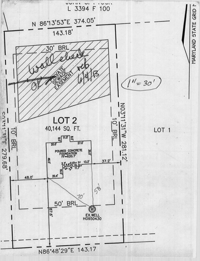
THIS WALL CHECK DRAWING CONTAINS A HORIZONTAL TOLERANCE IN ACCURACY OF 0.1' AND A VERTICAL TOLERANCE IN ACCURACY OF 0.2'
