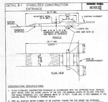
PIPE ALL SURFACE WATER FLOWING TO OR DIVERTED TOWARD THE SCE UNDER THE ENTRANCE.
