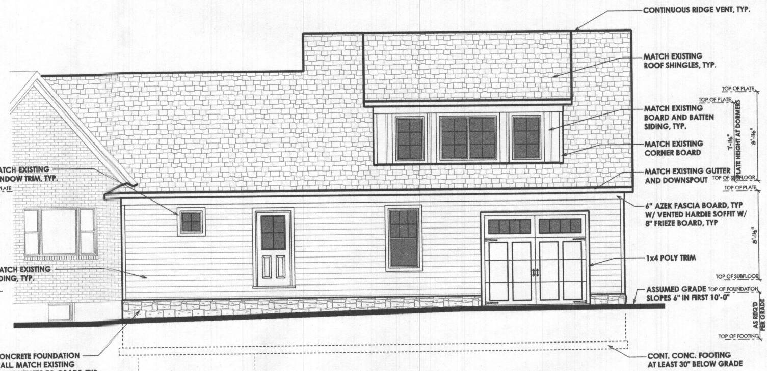
GARAGE - REAR ELEVATION
