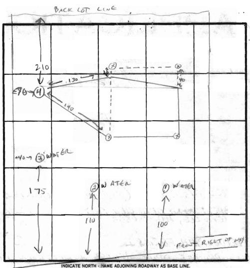
TEST - 1" DROP TEST NO. DATE DEPTH START TIME STOP STOP 6-10-83 3~ 8 WATE 11325 7 MIN 11132 4 11,25 5MW 11:20 12 MICA DRY - SAND
