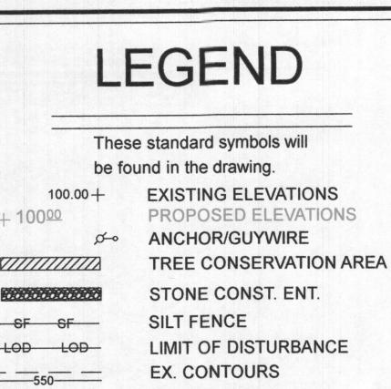
LOD LOD LIMIT OF DISTURBANCE UTILITY POLE -0-**EDGE OF PAVING** STREAM/CREEK EX. WOODSLINE SPECIFIC TREES PASSED PERCOLATION TEST HOLE SOILS LINE SEWAGE DISPOSAL AREA
