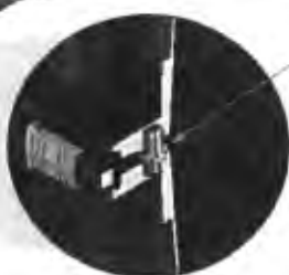
MID-SEAM CUTAWAY Reinforced water tight mid-seam gasketed connection
