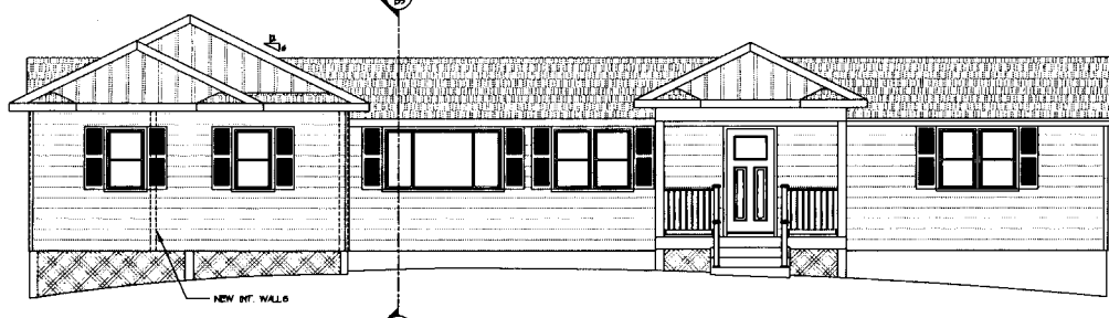
4 PROPOSED FRONT ELEVATION 1/8" = 1'-0"
